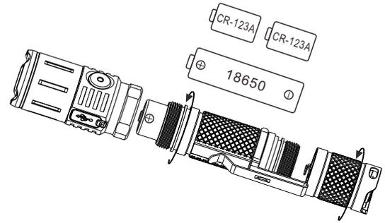
Powered by one 18650 battery or 2 x CR123A
