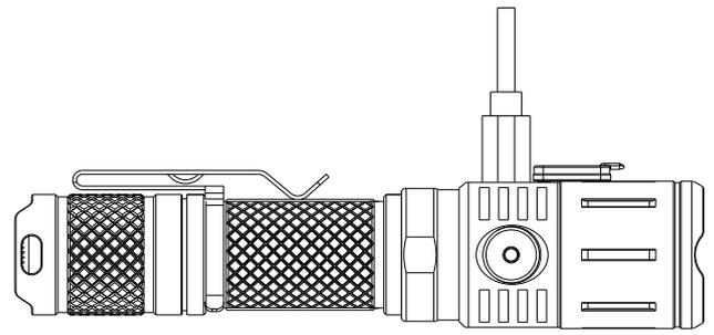
When the flashlight is in charging status, flashlight will automatically turn off and the red indicator at the switch position blinks once every 1.5 seconds.
